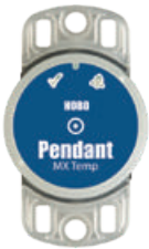
MX2201 Temperature Depth rating 100 ft
